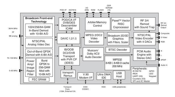
The BCM7115 is a single-chip set-top box device that combines the key aspects required for the next generation of set-top boxes, including cost-effective single-chip design, personal video recording (PVR), communication via DAVIC or other protocol, and support of all major global physical layer standards for worldwide deployment.
